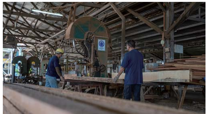
Trimming to specific sizes, in Tan Chee Seng Sawmill Perak, Malaysia. © Khairul Nizam Perak, Khairul Nizam
