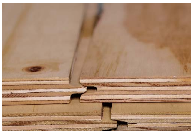
Tongue and Groove Product in Palmas PR, Brazil. Photo: Banco de Imagens Marini
