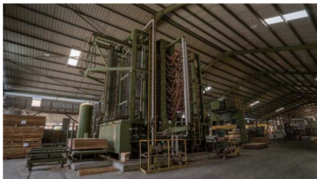
Hot pressing in Tan Chee Seng Sawmill Perak, Malaysia. Photo: Khairul nizam
